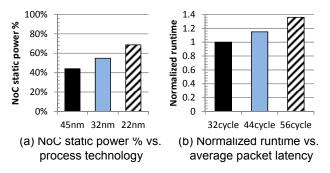
Figure 1: Need for reducing NoC static power without increasing packet latency.
